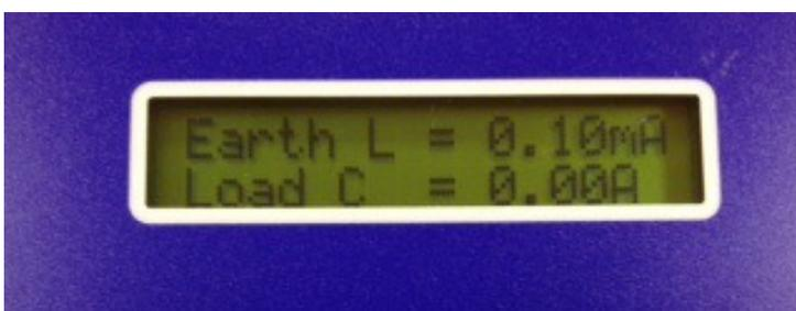
The meter continuously measures the Earth leakage and Load currents and displays this on the LCD.
