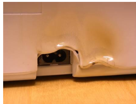
Damage to external casing
