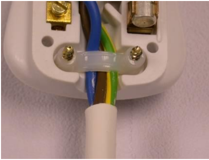
Cable not being gripped
