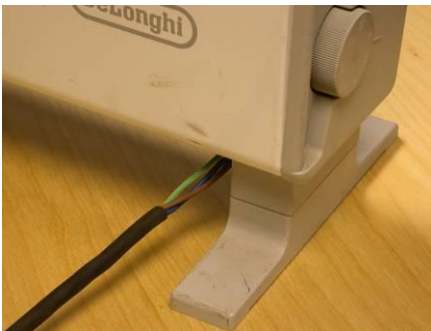
Cable not being gripped
