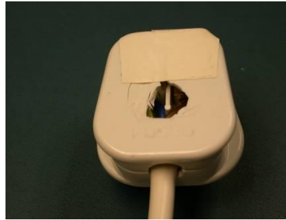
Damage to mains plug
