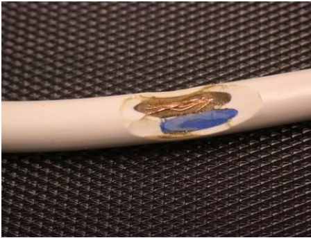
Damage to power cable sheath
