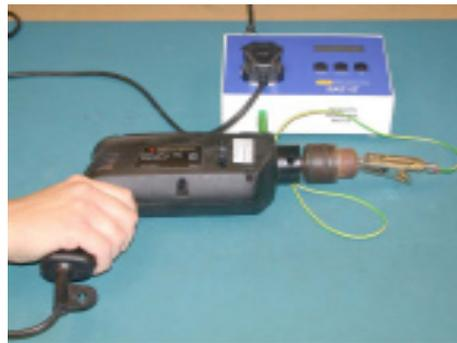
PAT-IT automatically assesses the test result for a pass or a fail.
