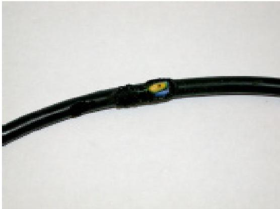
1a Damage to power cable sheath
