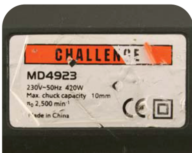
Fig 4.4: Rating plate on drill
