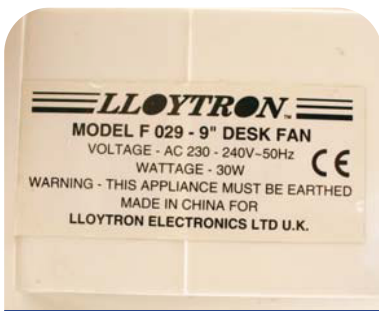
Fig 4.11: Electric fan: rating plate
