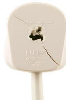
This shows a plug that has been damaged possibly because it has been dropped, or a piece of furniture has been moved against it. This is very common and is a
