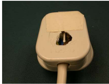
Damage to mains plug.
