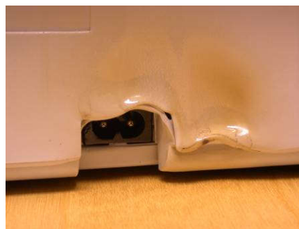
Damage to external casing.
