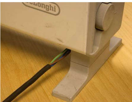
Cable not being gripped.
