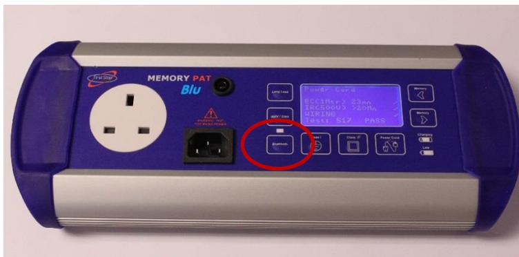
By default, the link will remain active for 1 hour. During the first 50 minutes, the LED will flash once per second. For the last 10 minutes of the hour, the LED will flash twice per second.
