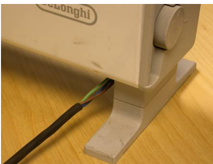
Cable not being gripped.
