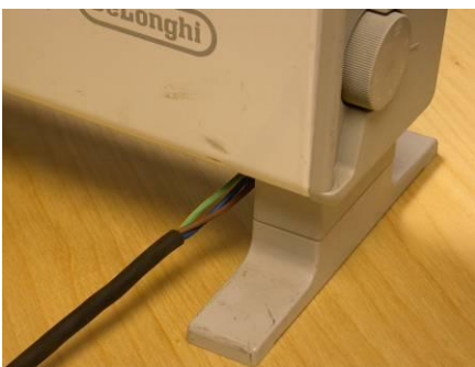
Cable not being gripped.
