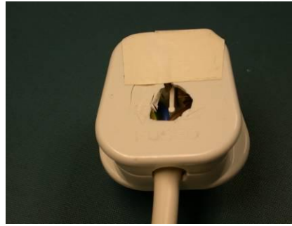
Damage to mains plug.
