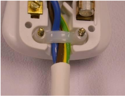
Cable not being gripped.
