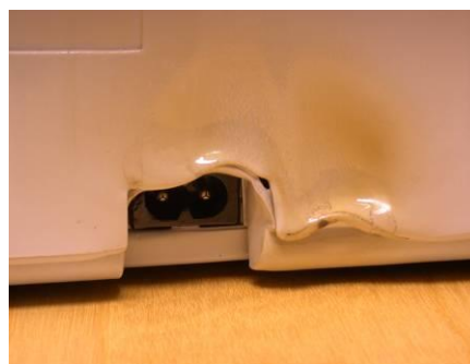
Damage to external casing.
